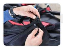
The pod is attached with zips either side of the harness, attach each side using the zips,
