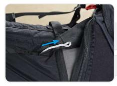
The speed line should then route through the protective cover located near the hip. Pass the line through the lower pulley housed within the protective cover and then through the upper pulley
