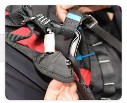
The cover can now be folded down to sit neatly on the bottom of the carabiner as shown.
