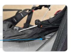
Route the line through the slit on the side panel of the harness making sure it is not entangled with any part of the harness structure.
