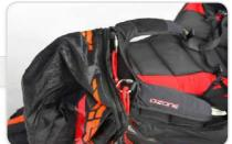
Attach the reserve parachute handle to the deployment bag using a larks foot knot. We recommend attaching the handle to the attachment point on the side of the deployment bag if it has one, otherwise it can be attached to the middle.
