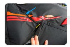
Close the bridle zip fully, the slider should be secured in the retainer by the left shoulder strap.
