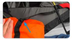
NOTE: You must check that the length between the handle and the container does not allow entanglement with the parachute lines.
