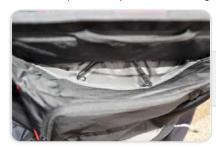
From inside the pod route the free end of the speed bar line through the speed bar retainer rings. These are found between the seat and ballast pocket. Ensure the elastics holding the rings are not twisted.
